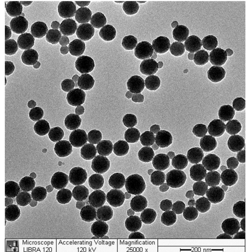
HRSEM and TEM of Slurry C2, colloidal silica, 50 nm
