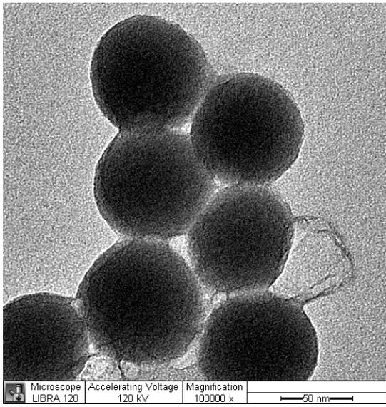
PS1 – dried colloidal silica (80 nm)
