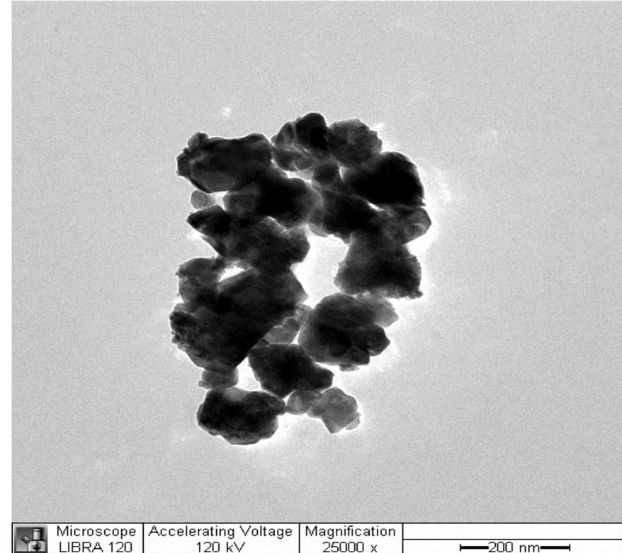
HRSEM and TEM of Slurry C4, ceria, 300-500 nm
