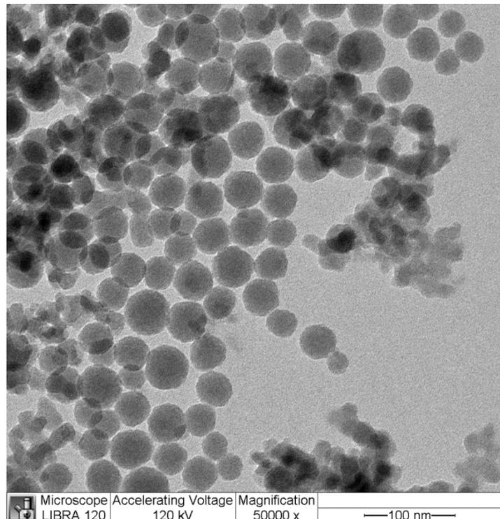
TEM of Colloidal Silica NPs in Slurry 1
