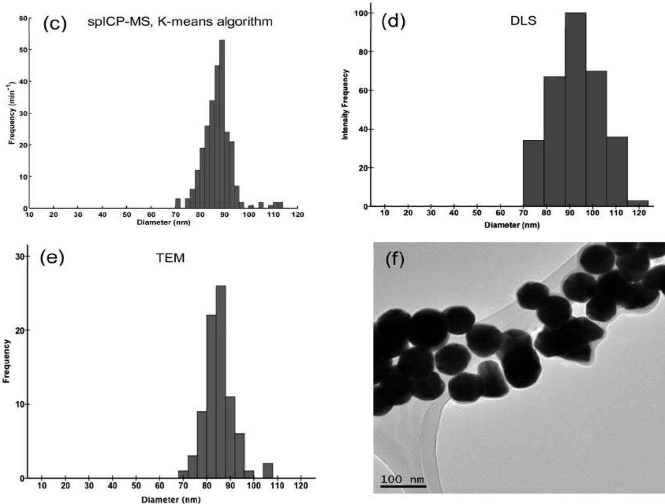
Fig. 2 (a–e) Particle size distribution histograms of BBI 80 nm AuNPs determined by different methods: (a) spICP-MS with  $4\sigma$  threshold signal processing, (b) spICP-MS with  $5\sigma$  threshold signal processing, (c) spICP-MS with K-means algorithm signal processing, (d) DLS, and (e) TEM based on counting >100 particles. (f) TEM image of AuNPs.
