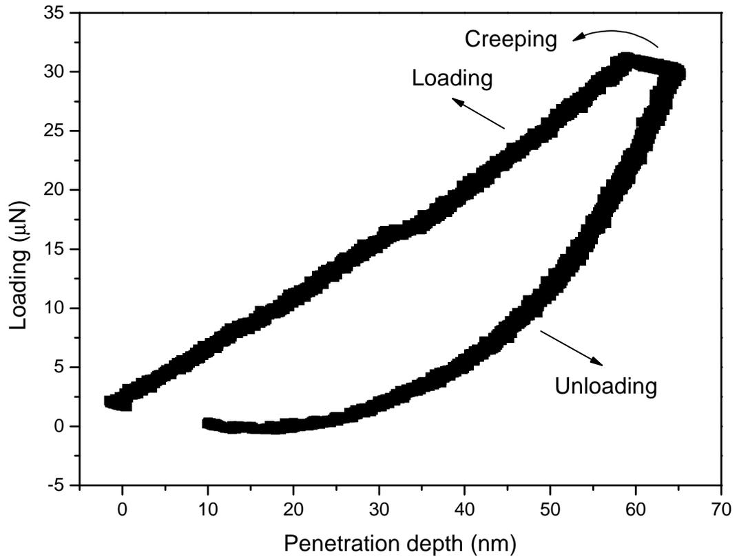
Figure 2. The loading and unloading profile used for nanoindentation measurement on the sacrificial layers which allows for the relaxation of viscoelastic effects in the polymeric materials.
