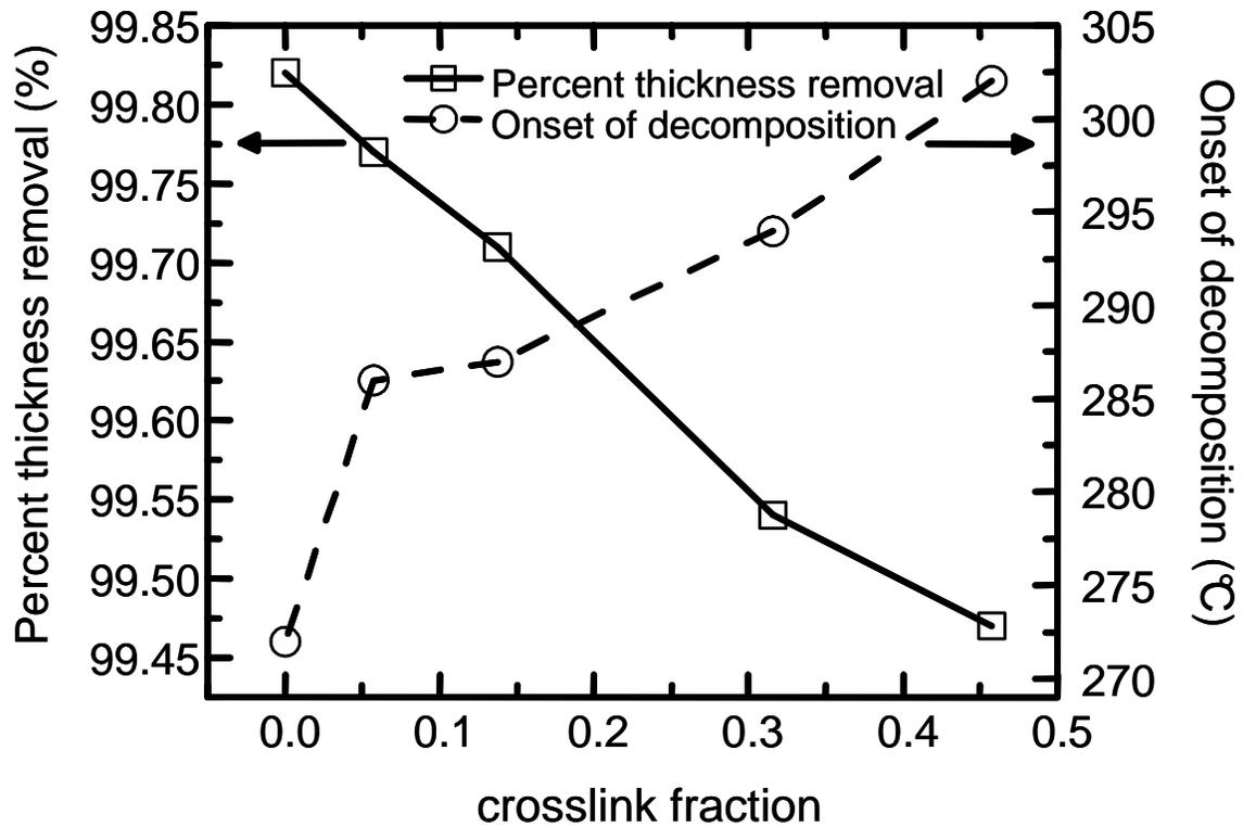
Figure 1. Thermal properties of iCVD films as a function of the crosslink density of the films. Left side axis corresponds to percentage of the sacrificial material remaining after annealing. The right side axis displays the temperature at which decompositions begins, representing the highest temperature which could be used from subsequent processing steps for integration of the sacrificial layer into an air gap structure.
