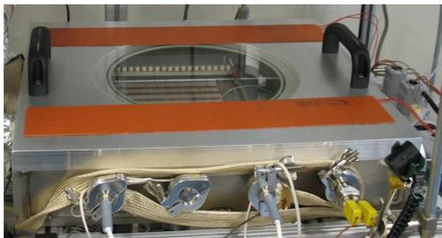
*Figure 2. New iCVD chamber capable of accommodating 300 mm wafers.*
