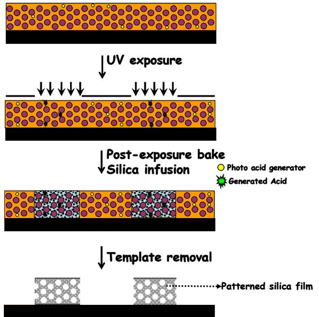
Scheme 1: Fabrication of patterned mesoporous silicate films from photo-patternable block copolymer films
