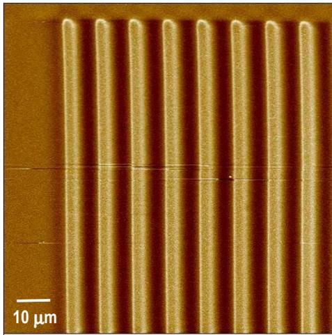
Figure 1: AFM image of patterned dielectric structures templated from P(IB-b-tbMA)
