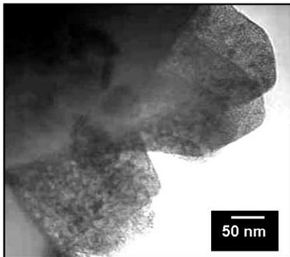
Figure 2: TEM image showing the Mesoporous structures present in the mesoporous silica film templated from P(S-b-tbocSt).
