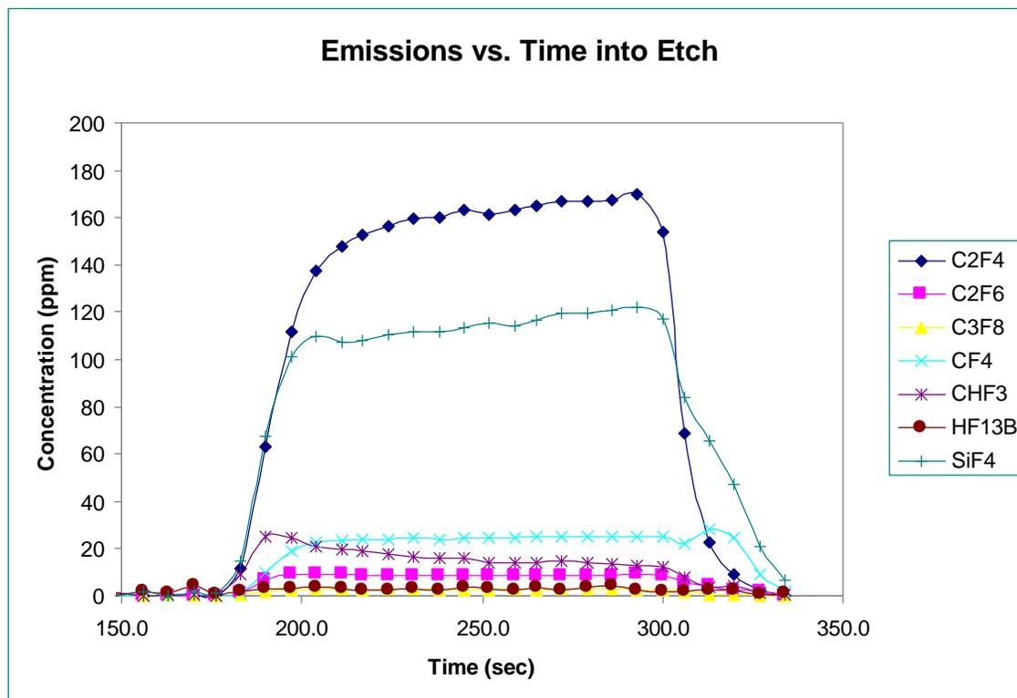
Significantly more  $C_2F_4$  being produced than  $C_2F_6$ ,  $CF_4$ ,  $C_3F_8$ , or  $CHF_3$ .
