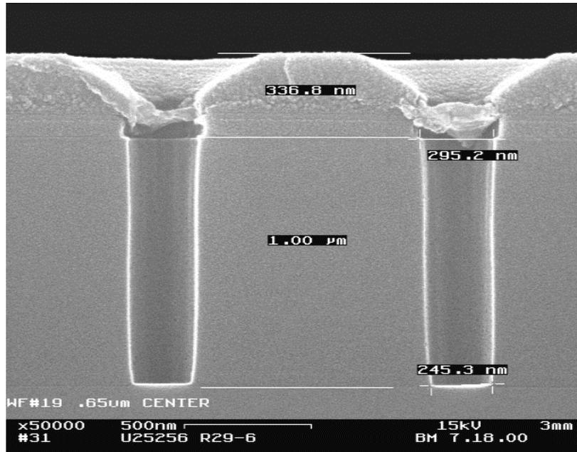
The breakthrough step is a less selective etch needed to breakthrough the silicon oxynitride ARC layer.
