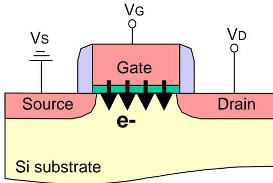
High device density & high speed transistor need high gate oxide capacitance and gate oxide scaling
