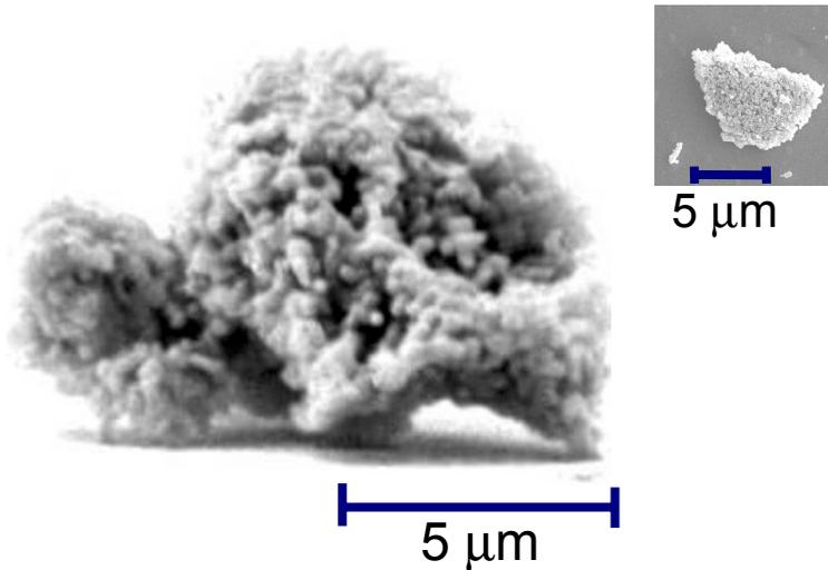
SEM of an alumina particle on a polished silicon substrate (15 KeV, 10000X, 87 degrees)
