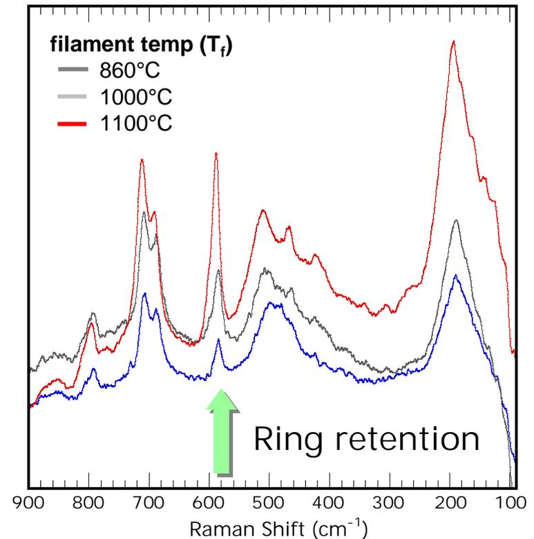
Filament temperature important control parameter
