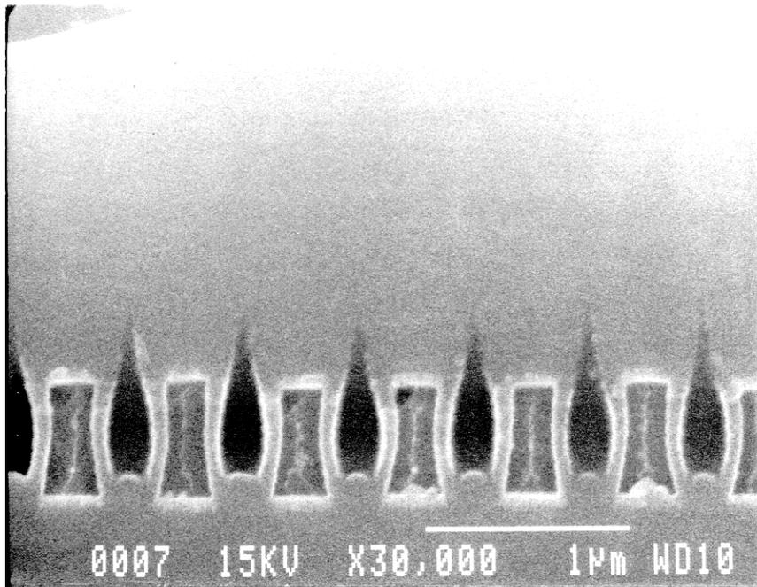
**Line/Space = 0.3μm/0.3μm**
