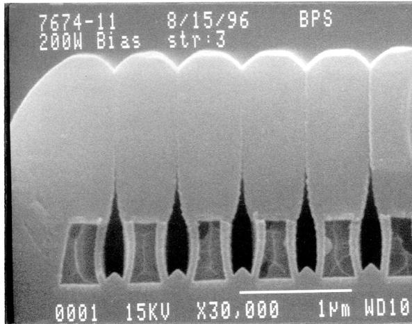
Line/Space =  $0.3\mu\text{m}/0.3\mu\text{m}$
