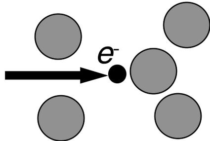
Metal atoms displaced by momentum transfer from electrons
