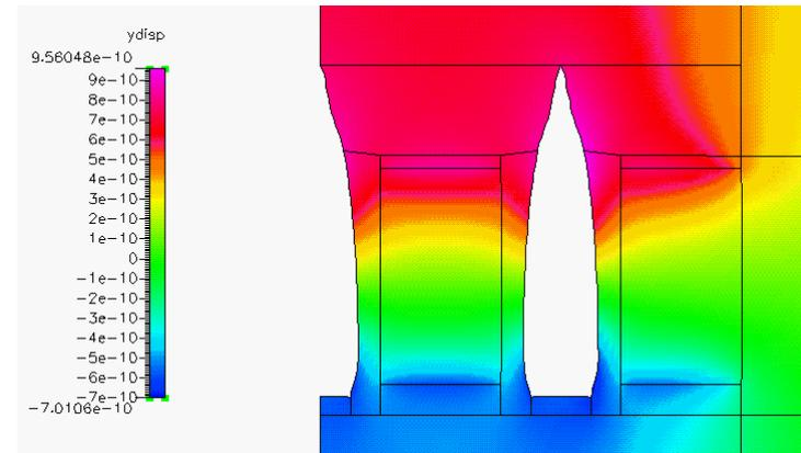
FEM simulation of y-displacement
