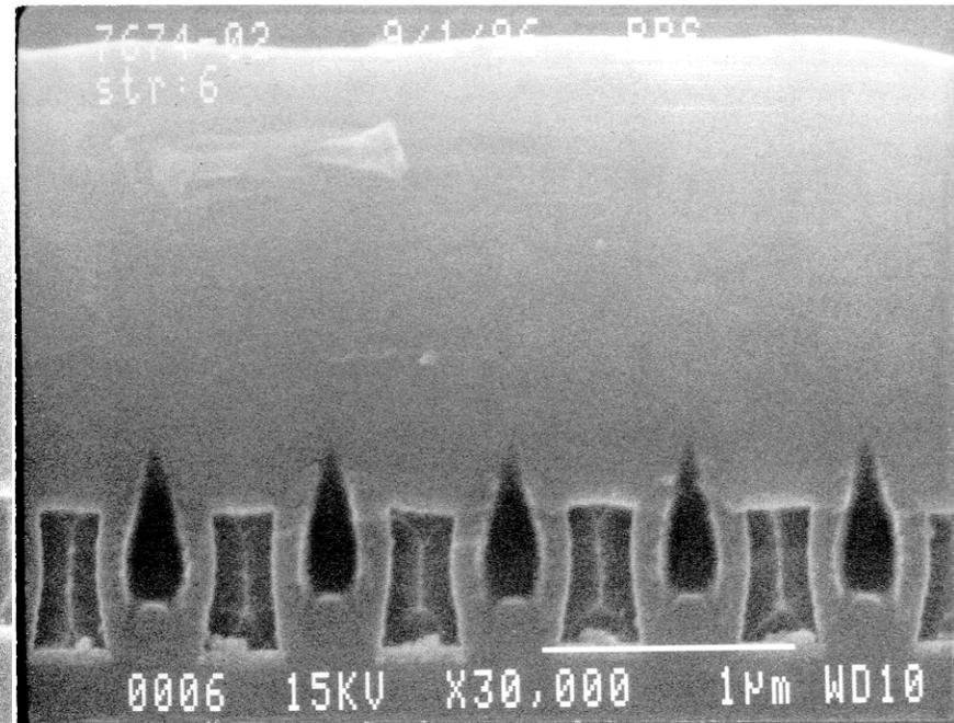
**Line/Space = 0.4μm/0.4μm**
