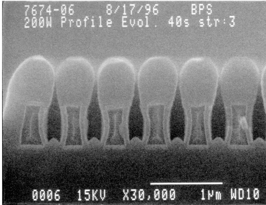
**Line/Space =  $0.3\mu\text{m}/0.3\mu\text{m}$**
