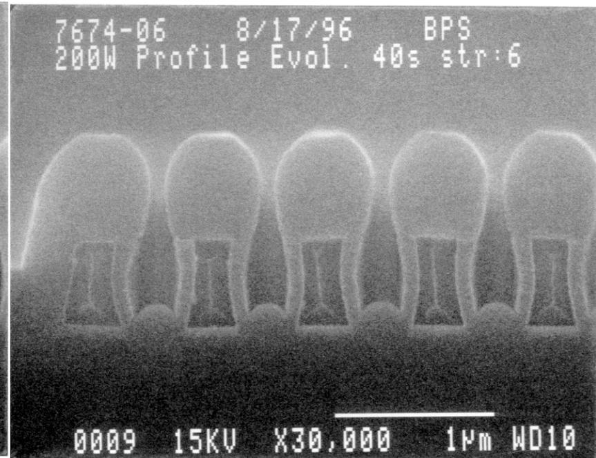
**Line/Space =  $0.4\mu\text{m}/0.4\mu\text{m}$**
