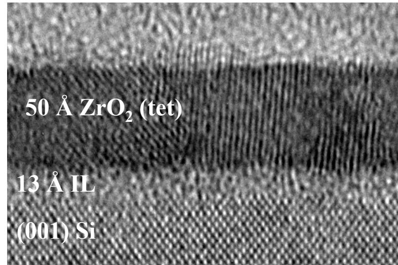
IL thickness > EOT ( $\therefore \kappa_{\text{IL}} > \kappa_{\text{SiO}_2}$ )
