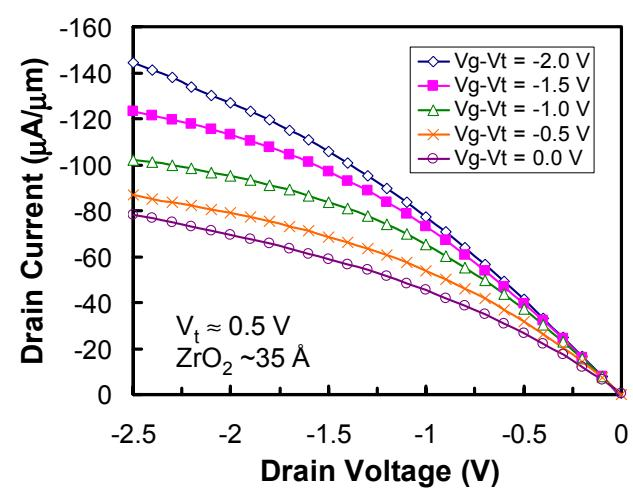
Output characteristics of a 2 μm
