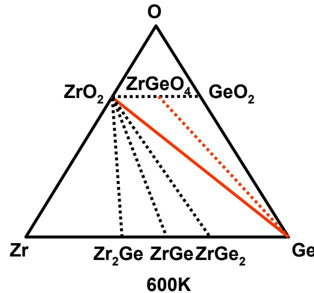
1.  $\text{GeO}_2 + \text{Zr} = \text{Ge} + \text{ZrO}_2$  (T=600K)
