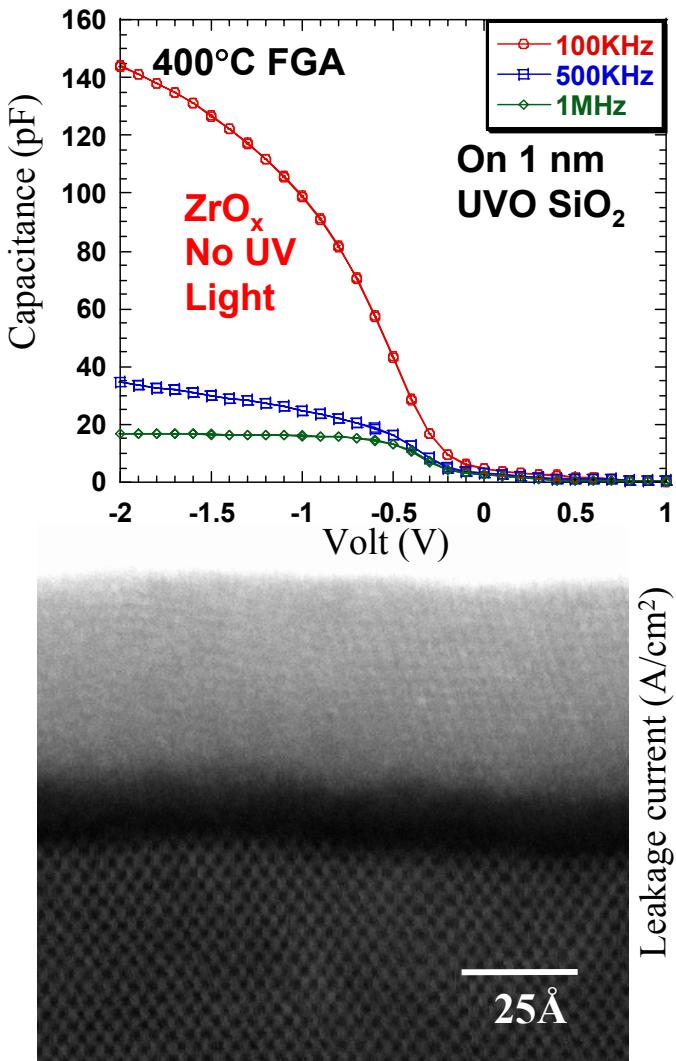
Polycrystalline  $\text{ZrO}_2$  film on thermal  $\text{SiO}_2/\text{Si}$
