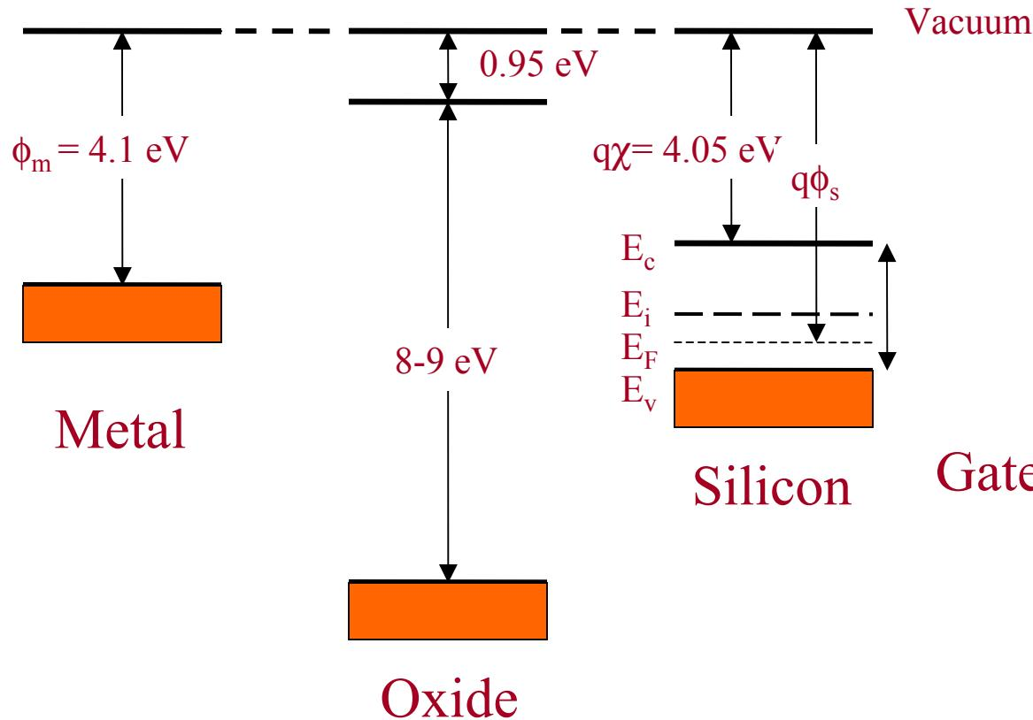
Schematic of the band diagram of a MOSFET
