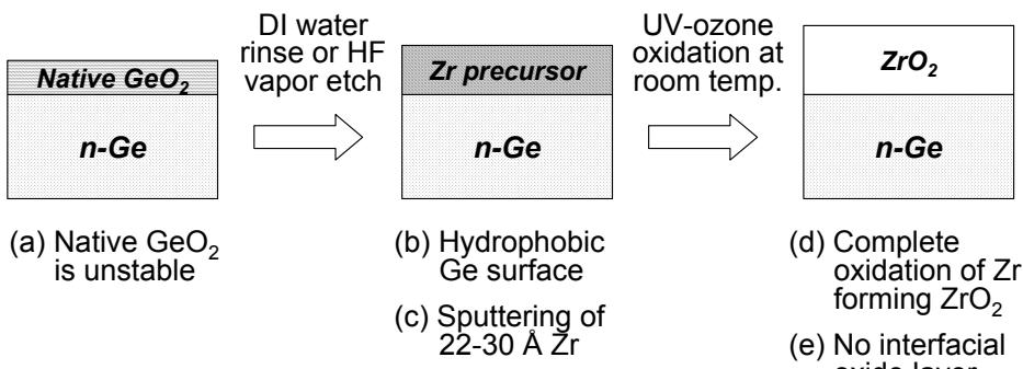
Interface layer-free room temperature  $\text{ZrO}_2$  deposition
