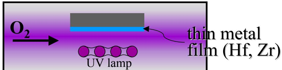
UV light supplies atomic oxygen and ozone to surface through the following reactions:
