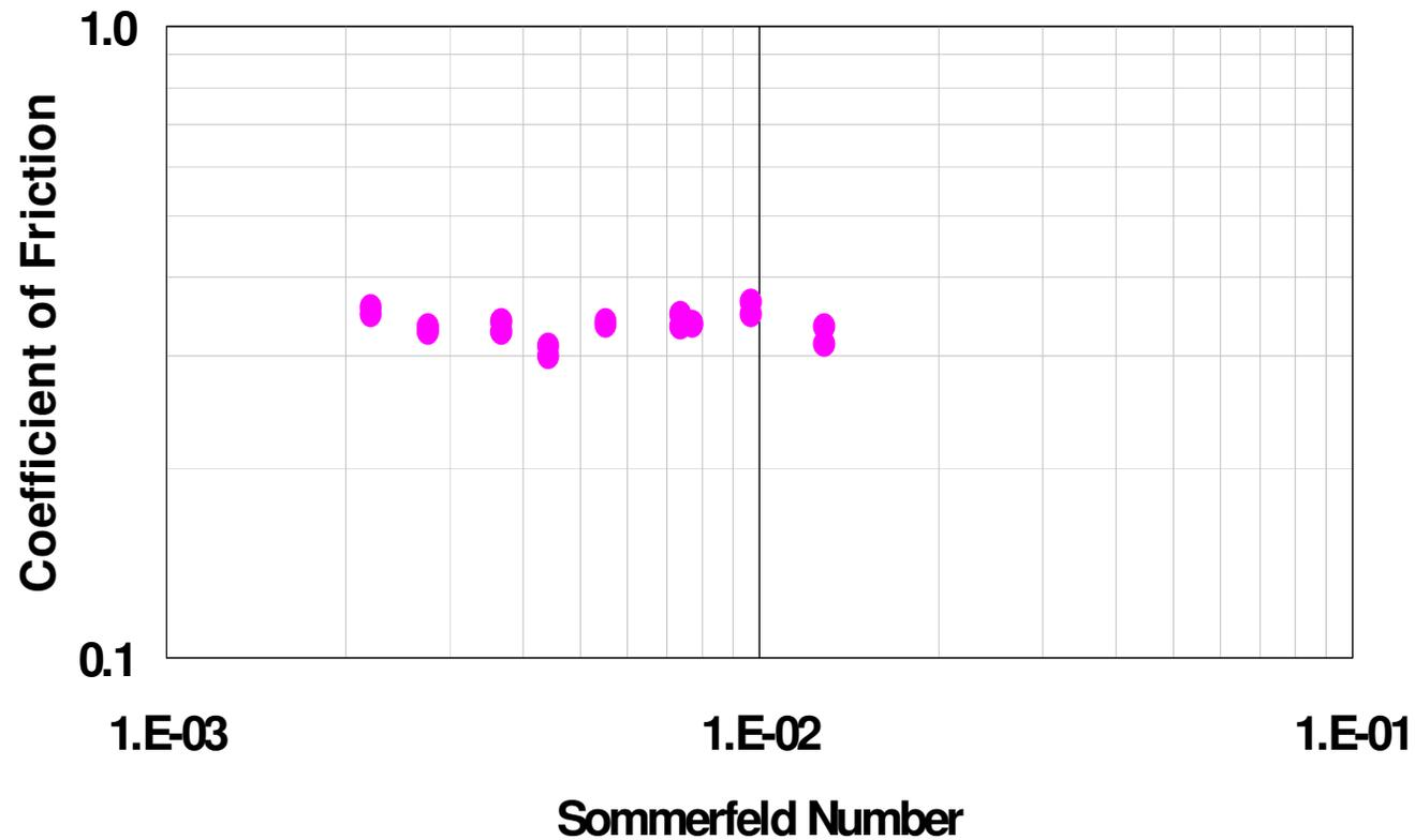
Tribological mechanism is 'Boundary Lubrication'
