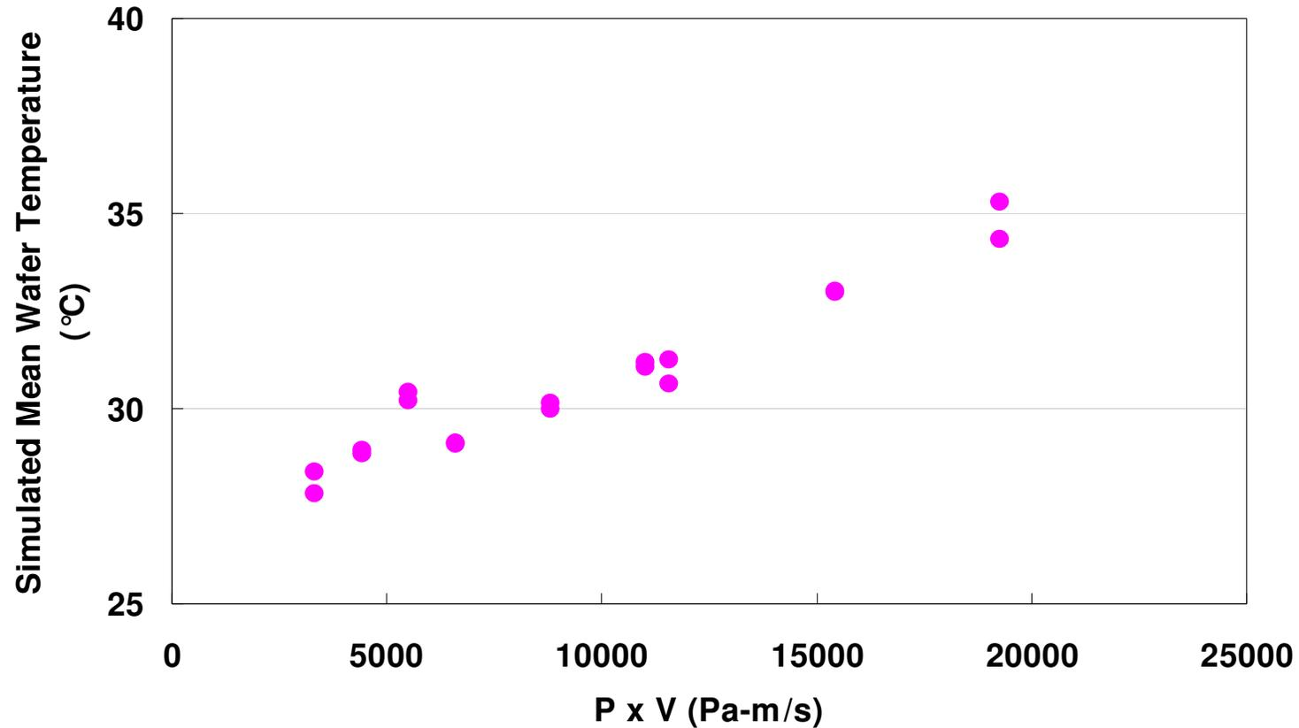
Simulated wafer temperature is higher than simulated/measured pad temperature, and has minimal effect on the significant increase in RR
