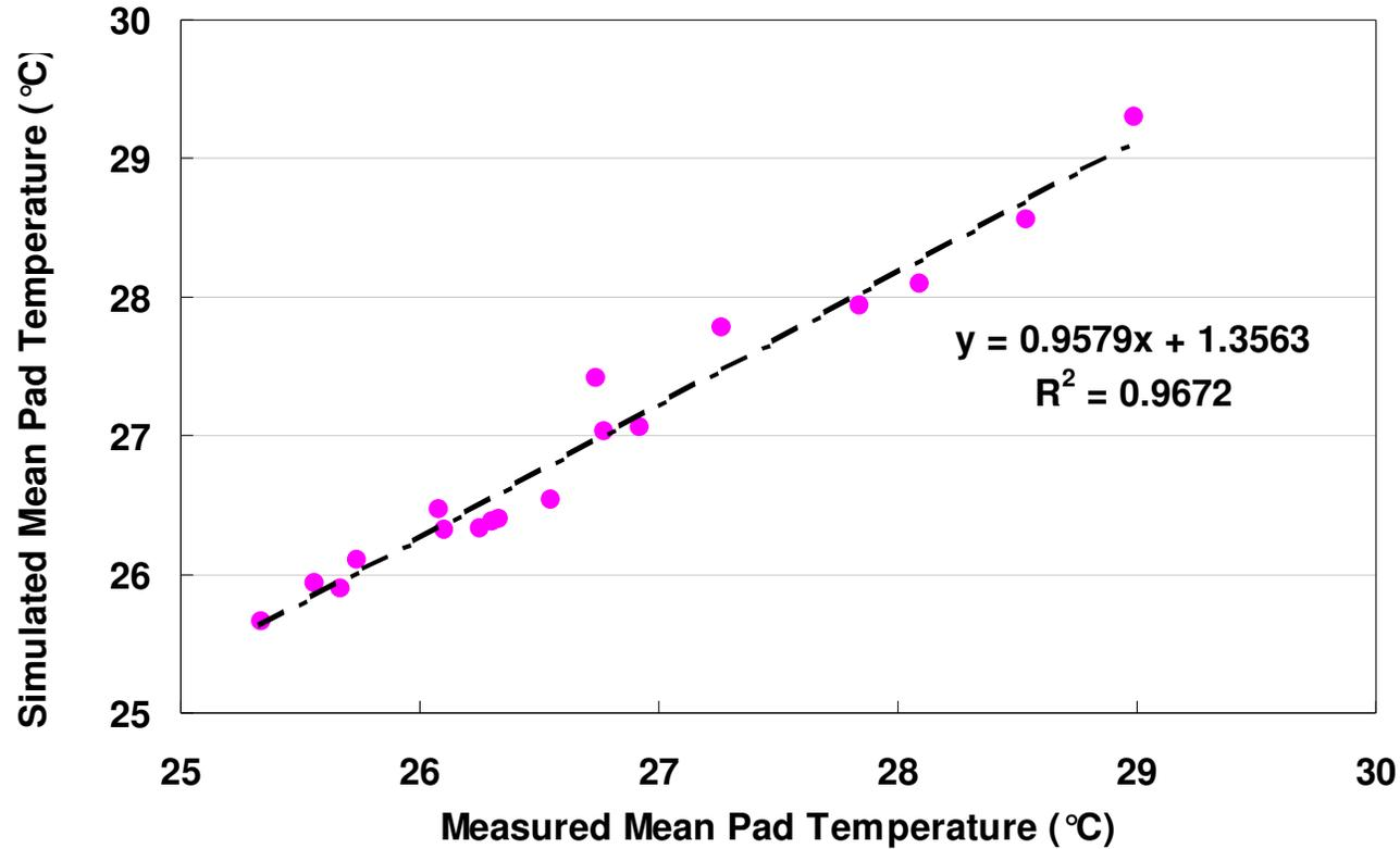
Simulated mean pad temperatures agree very well with the measured data.
