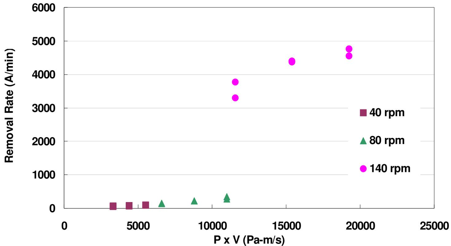
The non-Prestonian behavior is believed to be due to the presence of inhibitor in the slurry
