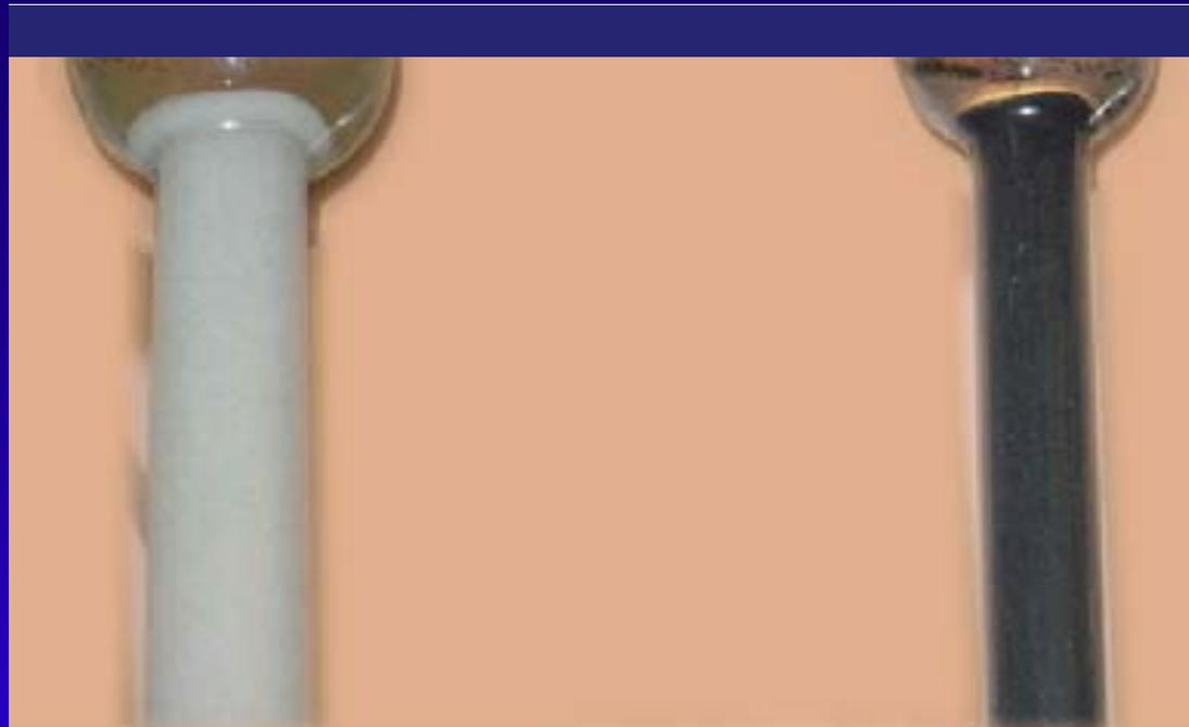
**Detail of the crystallization reactor during the first day (*left*) and after 5 days of operation (*right*) with an influent containing 5 mg Cu/l.**
