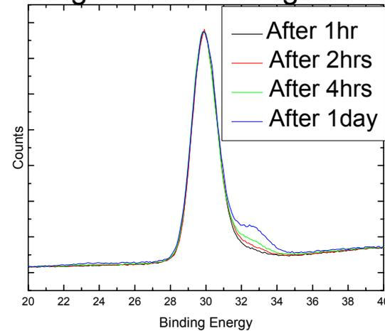
Nanowires grown with HCl during growth provide very stable passivation.
