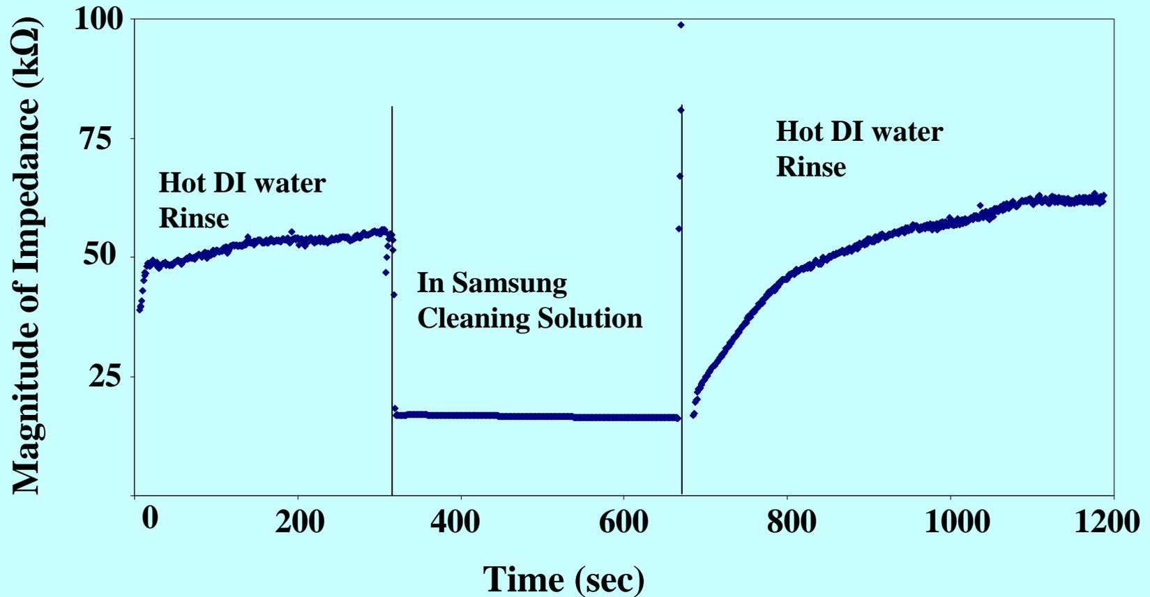
**ECRS can monitor cleaning of the polymer residue inside trench**
