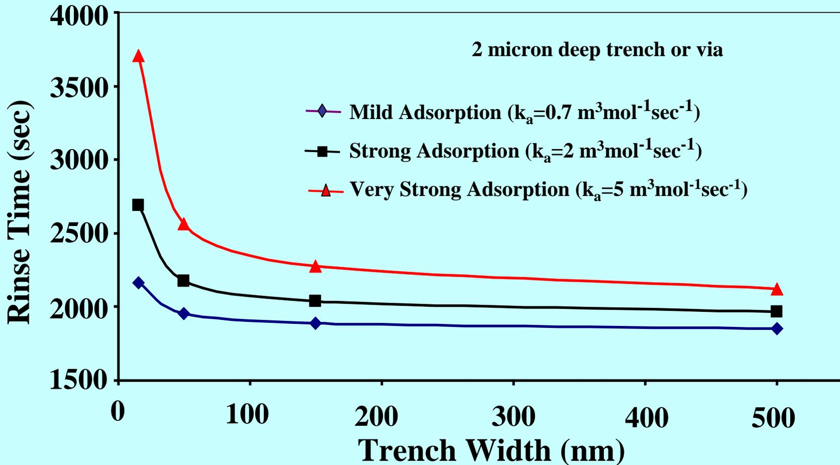
Rinse time to reach  $10^{12}$  ions/cm<sup>2</sup> on the surface of the trench.
