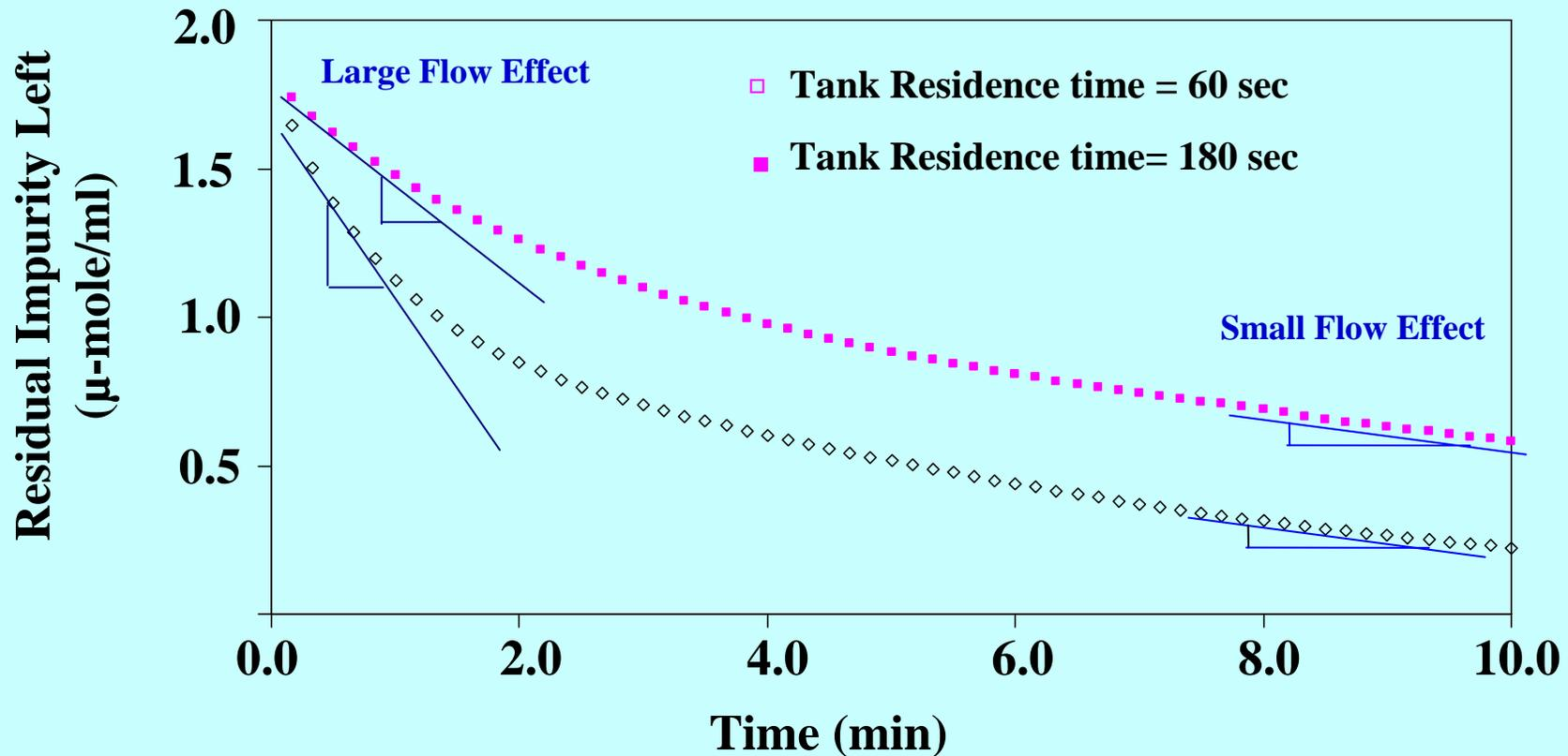
Large savings and water use reduction are possible with staged flow rate based on the proposed metrology.
