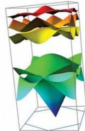
Bands of **negative slope** represent frequencies at which **negative refraction** will occur.
