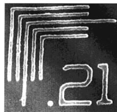
Figure 7. Features resolved using THPMA-b-F7MA copolymer using 193 nm exposure and scCO<sub>2</sub> development.
