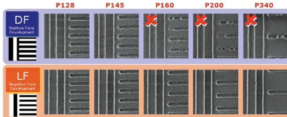
40 nm trenches with varying trench pitch
