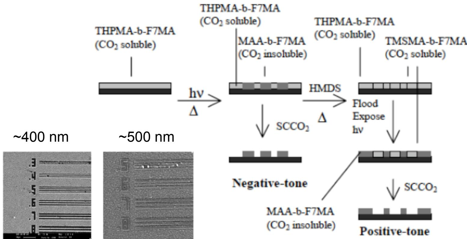
**Figure 2.** (a) THPMA-F7MA block copolymer resist exposed with 248-nm Nikon stepper and developed in scCO<sub>2</sub>; (b) sample processed after silylation, showing positive-tone patterns.
