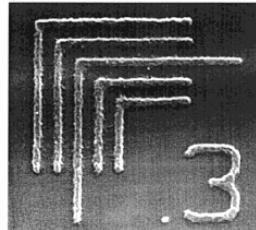
Figure 6. Features resolved using THPMA-b-F3MA copolymer using 193 nm exposure and scCO<sub>2</sub> development.
