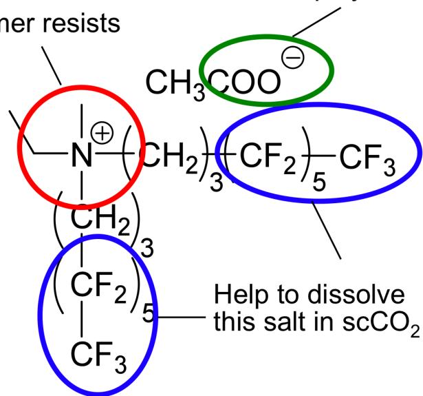
Deprotonate from OH and/or COOH in polymer resists
