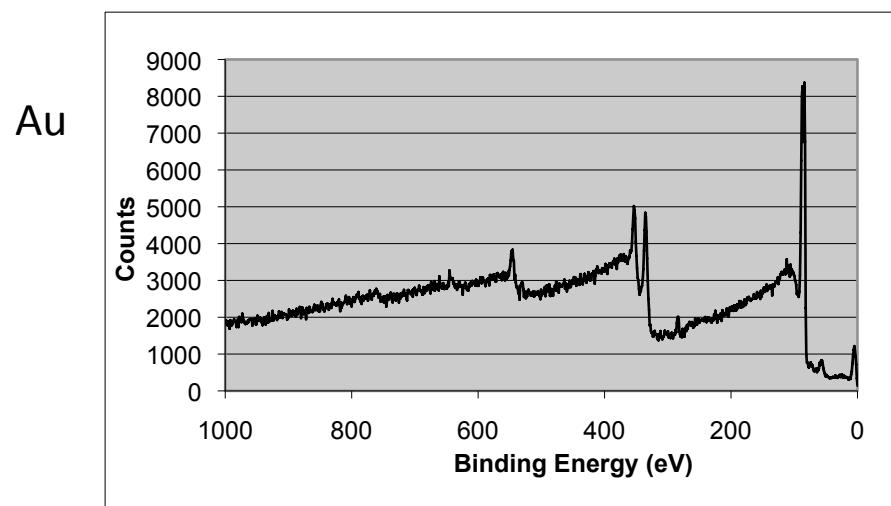
Au with residue-cleaned under  $\text{CF}_4$  for 30 s
